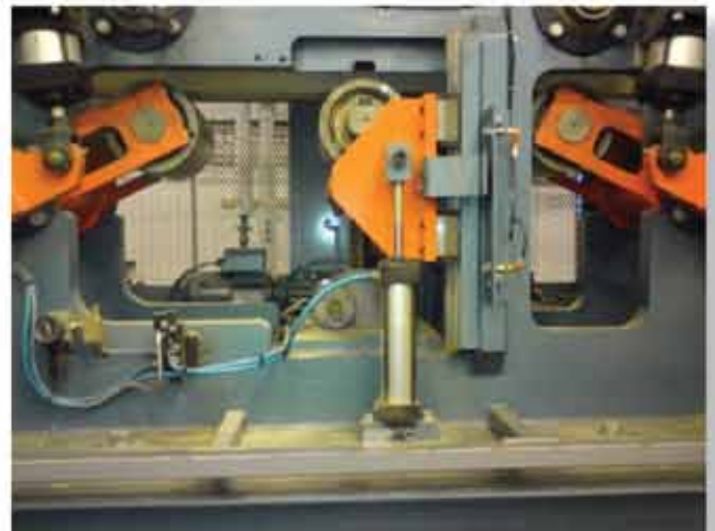
View of upward deflection unit in operation
